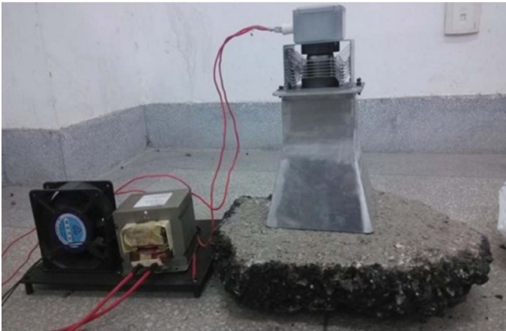
Figure1 - Experimental prototype of RF Asphalt heating process [2]
