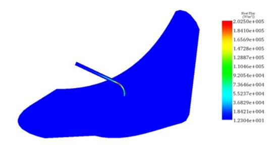
Figure 8 - Heat flux distribution at 2.45 GHz
