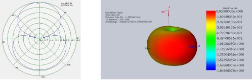
Figure 3 - 2D and 3D radiation patterns of the dipole antenna at 2.3 GHz
