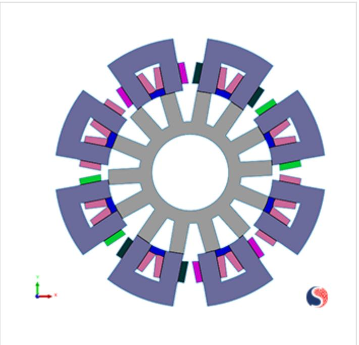
Fig. 2. (b) Permanent Assisted 4-Phase 16/14 SRM Motor
