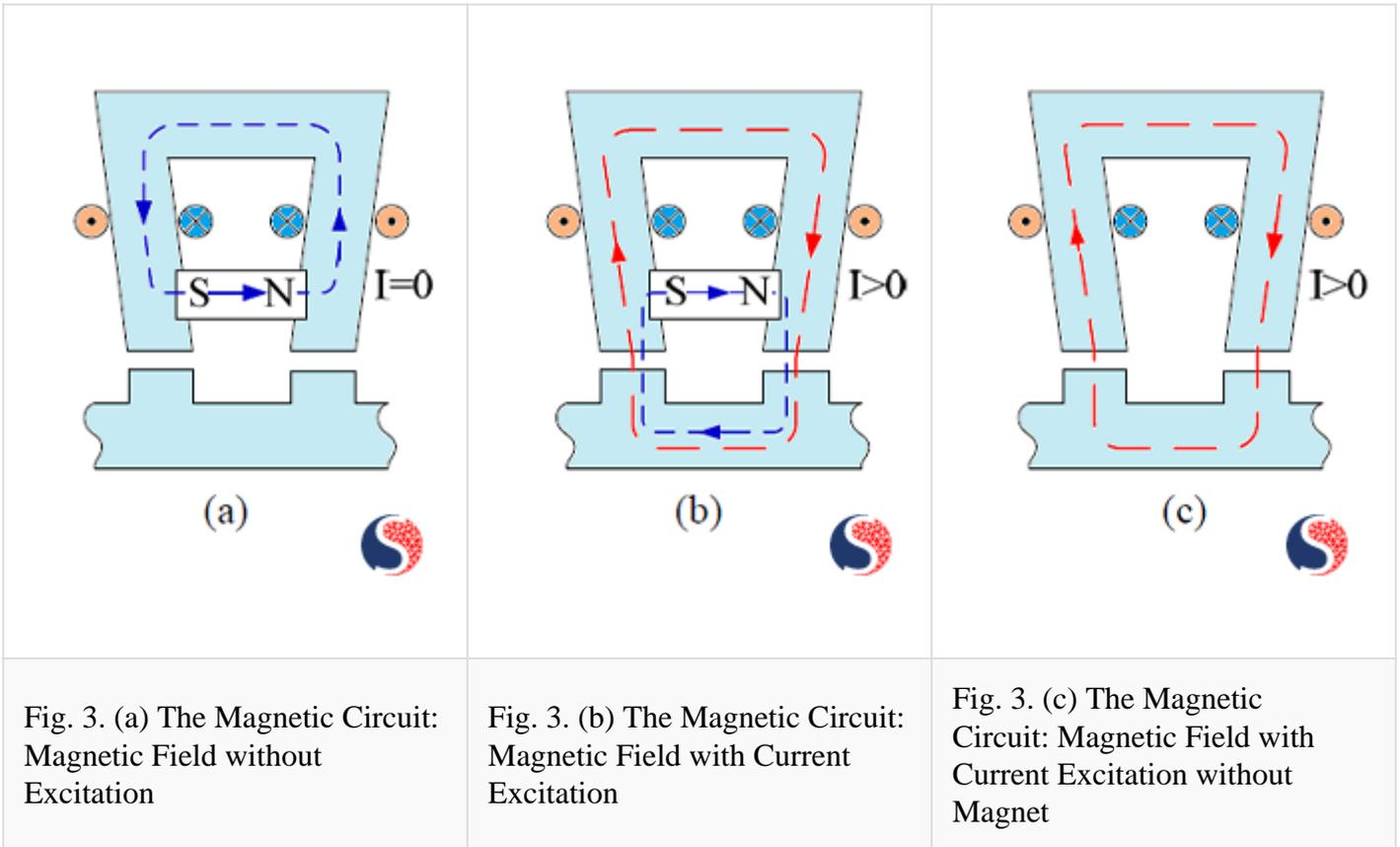
Fig. 3. (a) The Magnetic Circuit: Magnetic Field without Excitation
