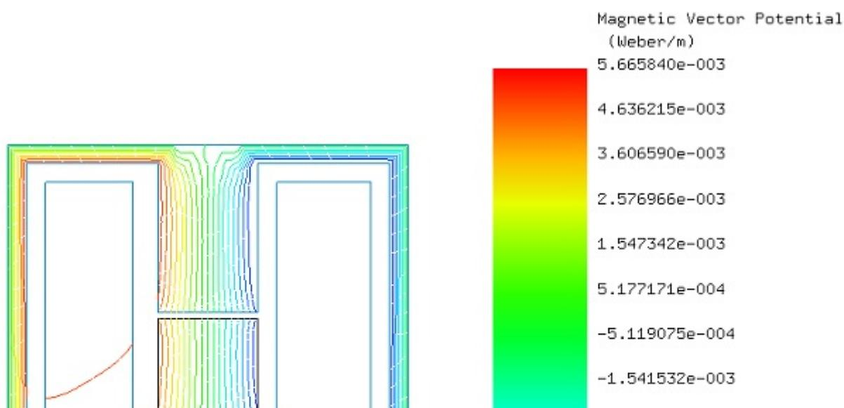
**Figure 6 - Flux lines of the magnetic vector potential.**
