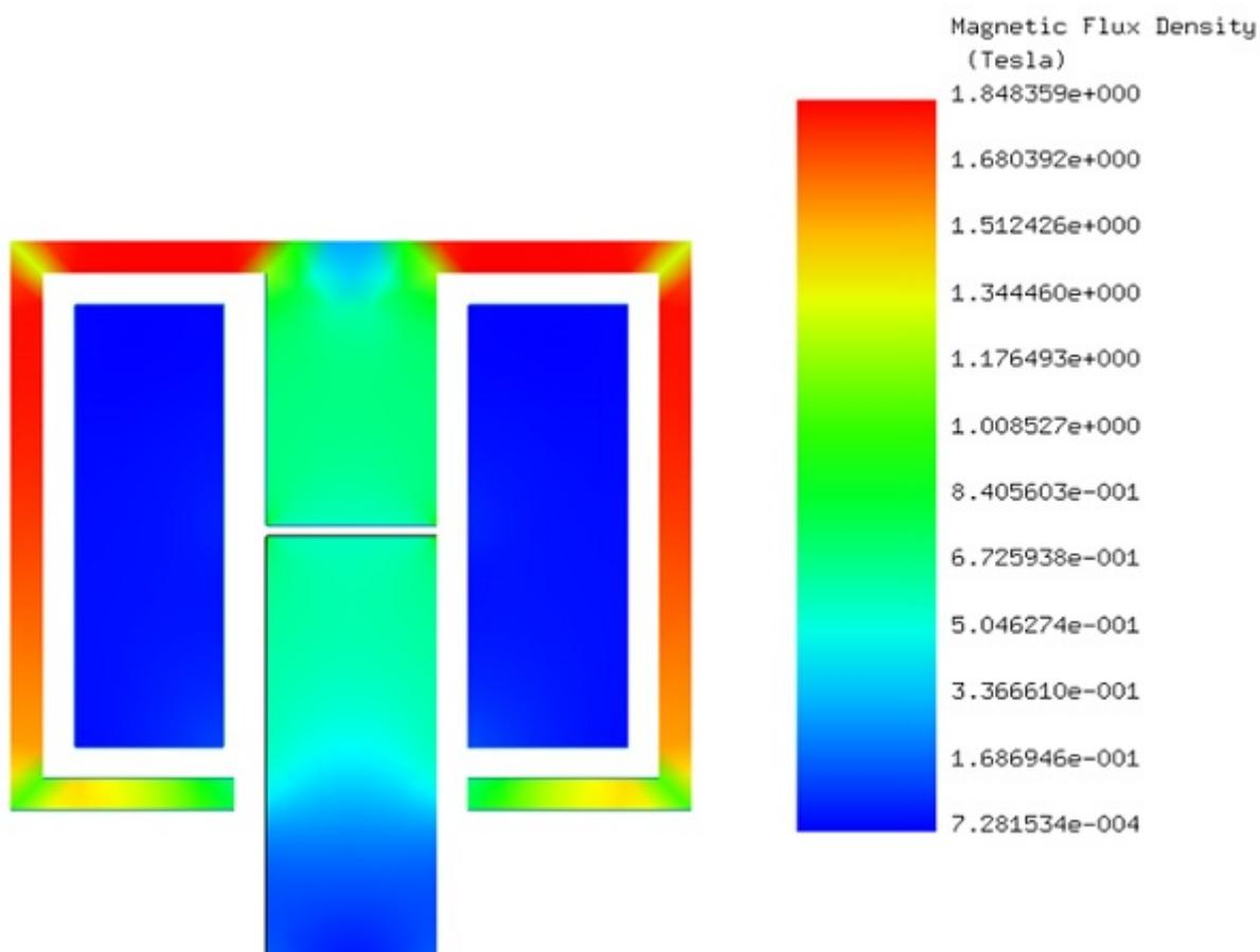
*Figure 5 - Fringe plot of the magnetic flux density.*
