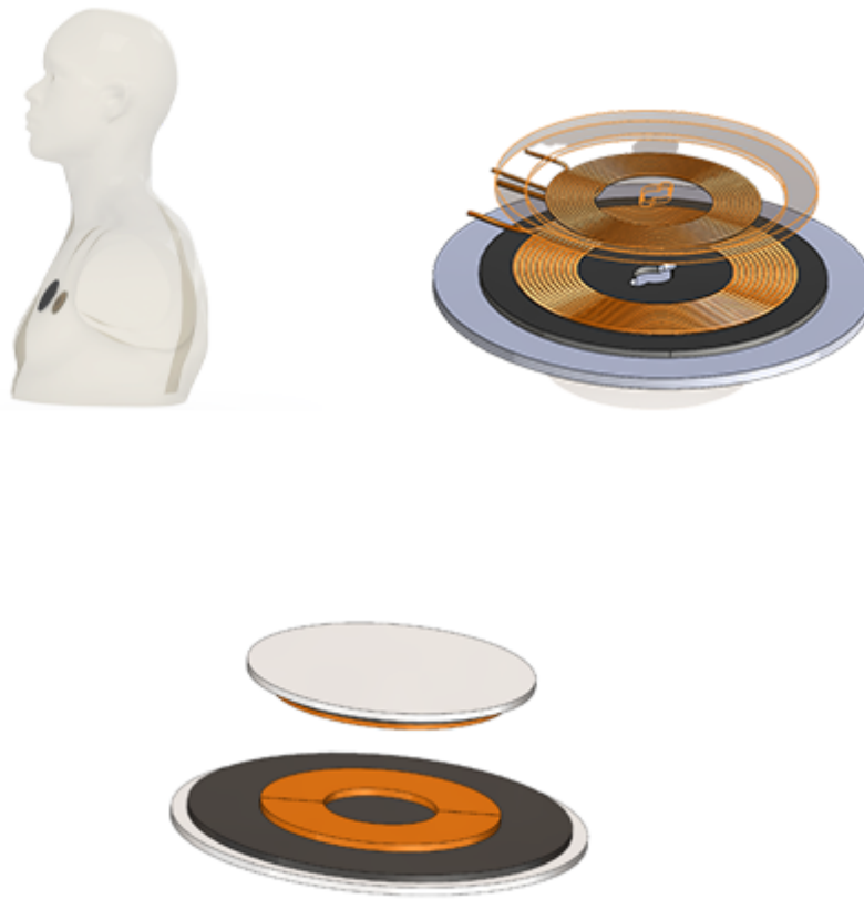
Fig. 2. 3D Model of WPT Design used in Pacemaker Application
