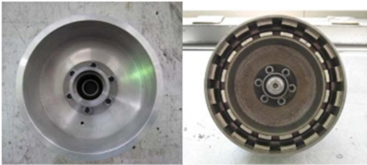
Figure 1 - Prototype of the DSPM eddy current coupler [1]
