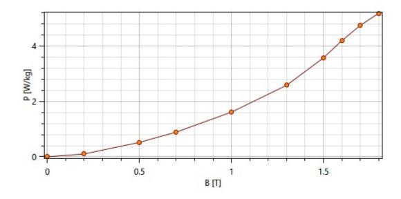
Figure 2 - Core BP Curve
