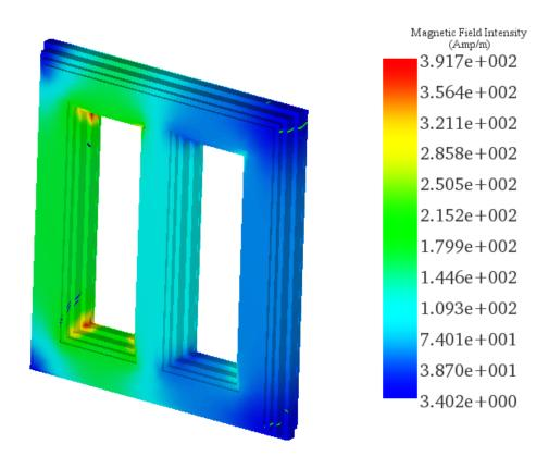
Figure 5 - Magnetic field intensity in the transformer
