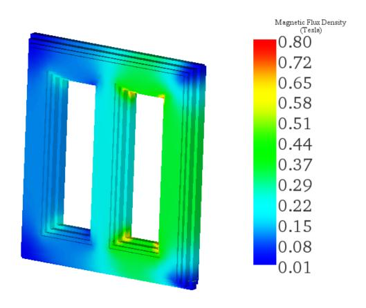
Figure 4 - Magnetic flux density in the transformer
