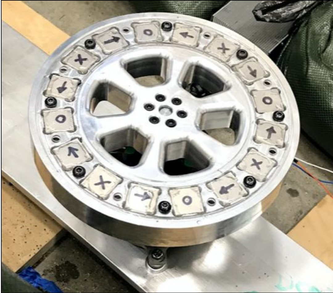
Figure 3: The machined wheel with installed magnets.
