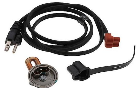
Figure 2: Engine block heater resistive element (copper-colored unit), extension cord to grille, and extension cord prongs cover [10]
