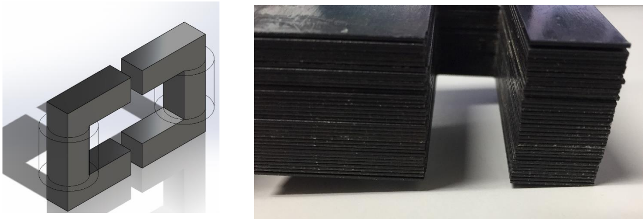
Figure 8: (Left) basic CAD model of core; (Right) stacked laminated layers to reduce eddy currents
