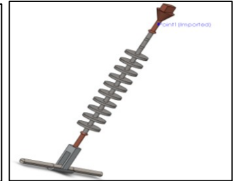
Figure 40: Insulator with 10 discs
